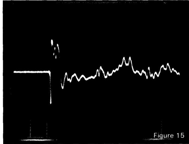
are in the same polarity. Figure 14 shows the response. Figure 15 is the same system but with the tweeter polarity opposite that of the woofer. Figure 16 is the resulting response showing a substantial dip at the crossover frequency. Figure 17 again shows a comparison between the system in phase and out of phase.
